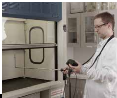
Plug and play thermoanemometer probes enables use in multiple applications.
