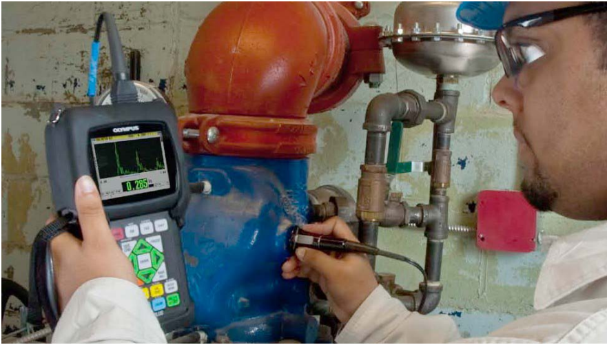
Figure 1-1 Measuring thicknesses with the 38DL PLUS
