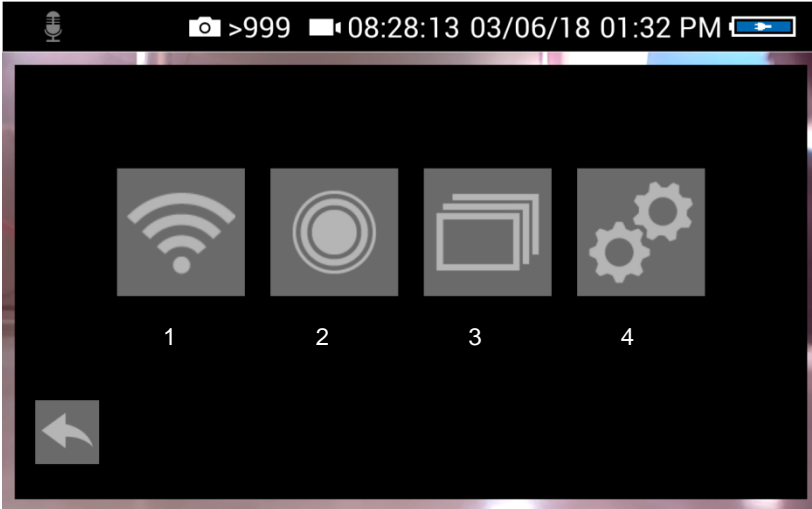
Fig. 30: System menu with submenus WLAN (1), Locator detection (2), Image and video gallery (3) and settings (4)
