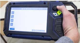
Fig. 14: With the handle pulled out it is possible to hold and operate the monitor with one hand.
