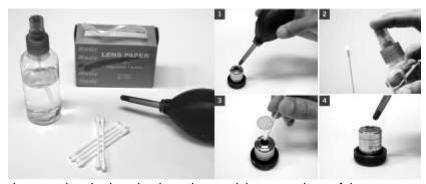
by screwing the lens back on the revolving nosepiece of the microscope.
