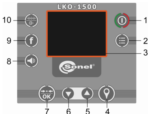
Fig. 9 Design and labeling of receiver buttons LKO-1500
