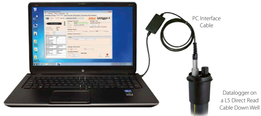
Figure 2-7 Datalogger and L5 Direct Read Cable Connected to PC Using a PC Interface Cable
