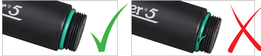
Figure 10-25 Levellogger O-ring Damage
