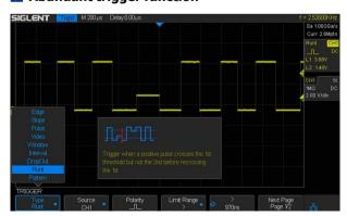
SDS1000X/SDS1000X+ has a wealth of trigger modes, including Edge, Slope, Pulse, Video, Windows, Runt, Interval, Time out (Dropout), Pattern, IIC, SPI, UART/RS232, LIN, CAN
