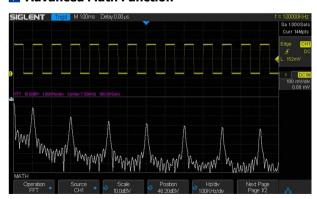
In addition to the traditional (+, -, X, /) operation, SDS1000X/ SDS1000X+ oscilloscopes supports FFT, integration, differentiation, and square root operations.
