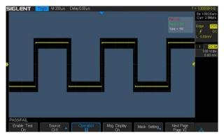
The SDS1000X/SDS1000X+ utilizes a hardware-based Pass / Fail function, performing up to 40,000 Pass / Fail decisions each second. With easy to generate user-defined test templates, the SDS1000X/SDS1000X+ compares the current measured trace to the template mask trace making it suitable for long-term signal monitoring or automated production line testing.
