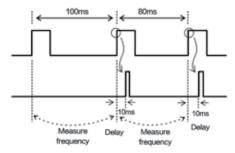
If the current period of external trigger input changes, the time of the flash is not accurate, because the time is calculated based on the previous measurement period.
