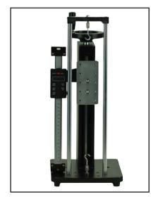
Stand with Optional Tensile Frame and Digital Scale
