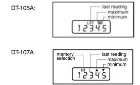
To fill all three memory spaces, unit must operate for about 5 seconds. If any of the above memory readings are missing, unit must operate a few seconds longer.
