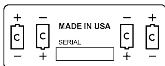
Battery installation diagram / Serial number label
