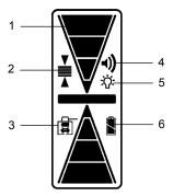
Grade Indication Arrows - 11 individual channels of grade display. Arrow size increases as distance away from on-grade increases.
