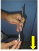
remove rotor stator and teflon bearing
