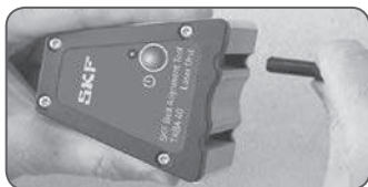
Fig 2 Fitting or removal of V-guides
