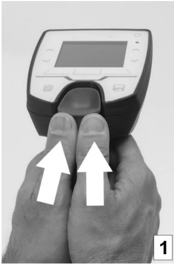
Fig. 9: Dismounting the pump
