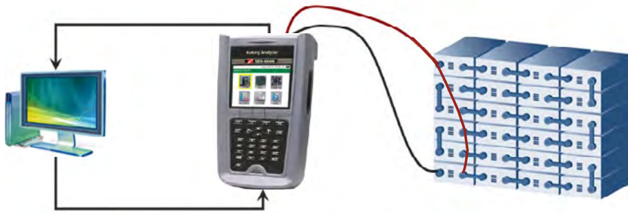
Battery resistance testing
