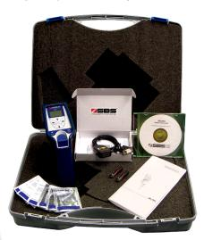
The SBS-2500 offers the ability to test the specific gravity and temperature of lead acid or nickel cadmium batteries within seconds. The unit is able to take readings between the range of 0.0000 to 2.0000.
