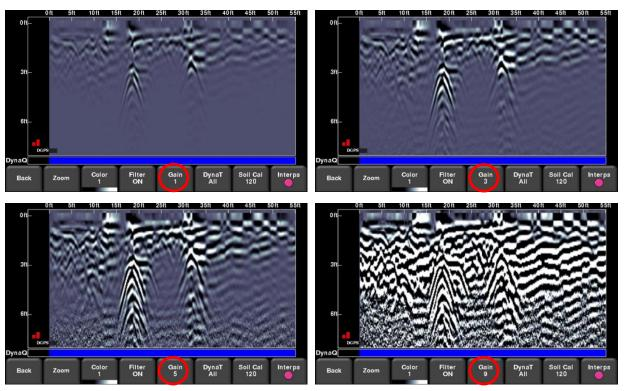
Figure 8-11: Varying the Gain
