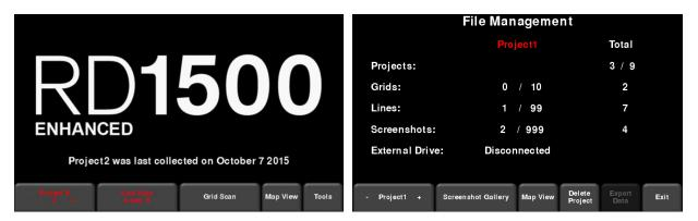
Figure 11-2: Accessing Map View from RD1500 Enhanced, either from the a) Main screen or b) File Management menu
