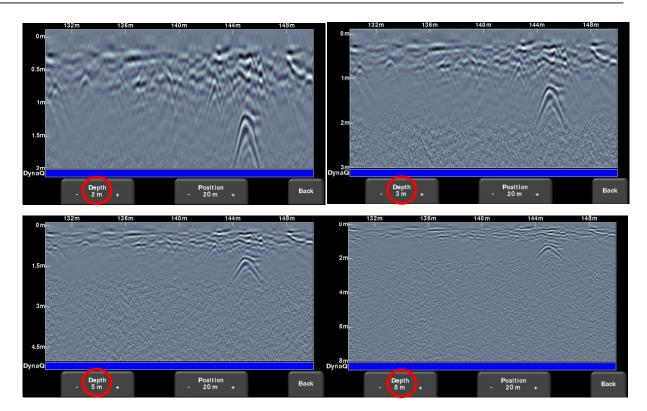
Figure 8-7: Varying displayed depth
