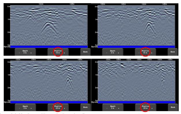
Figure 8-8: Varying position, or horizontal scaling
