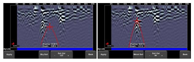
Figure 8-13: Adjusting Soil Cal, a) initial screen. b) moving the red hyperbola over a hyperbolic response from a subsurface target
