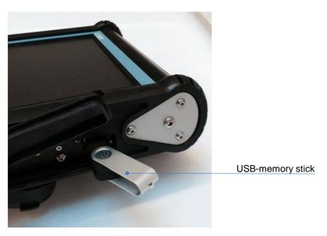
Figure 13-1: Insert a USB memory stick into the USB port on the Display Unit to export data.
