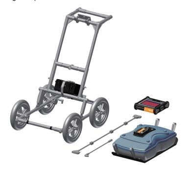
Attach the GPR Sensor to the Cart using the Sensor Support Straps. Ensure the Sensor is oriented the correct way with the connections toward the back of the Cart. Using the Sensor Support Straps, adjust the height of the Sensor so it is 1-2 cm ( $\frac{1}{2} - \frac{3}{4}$  inch) above the ground. The best way to get a uniform Sensor height is to place a couple of sheets of thick cardboard, particle board or Styrofoam on a level surface under the sensor before securing the Sensor Support Straps.
