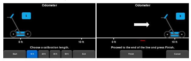
Figure 6-12: Odometer Test. Image on the left shows the screen where the user must select a distance. The image on the right instructs you to move that distance then press Finish.
