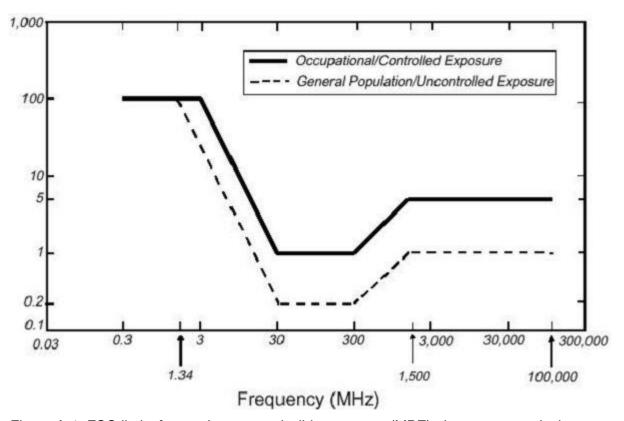
Figure A-1: FCC limits for maximum permissible exposure (MPE) plane-wave equivalent power density mW/cm<sup>2</sup>.
