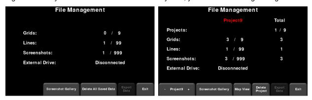
Figure 6-6: a) RD1500 system on left, displays the total number of lines, grids and screenshots saved on the system. b) The RD1500 Enhanced system on the right displays the lines, grids and screenshots for a given project in the middle column. The right column displays the total for each that are saved on the system.
