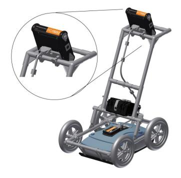
Attach the Odometer and Battery Cables. The Odometer Cable connects to the closest receptacle on the Sensor. Attach the Battery Cable to the Sensor and the Battery. The system is now set up and ready to use.
