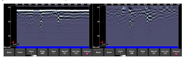
Figure 8-10: Left image shows **Filter On**, while the right shows the same data with the **Filter Off**.
