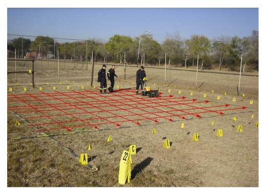
Figure 9-2: Example of a grid survey. The red lines are superimposed just to illustrate the concepts.
