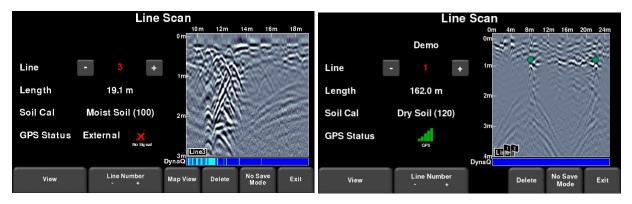
Figure 8-2: Line Scan mode, showing a line that was previously collected (a) RD1500 on left, (b) RD1500 Enhanced on right. The RD1500 has the MapView option on this screen.
