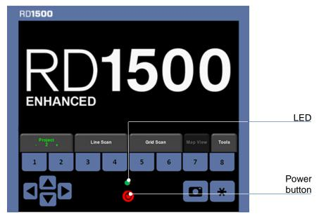
Figure 5-1: Front of Display Unit
