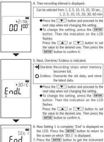
7. Press the **ENTER** button to get the instrument ready for a measurement.
