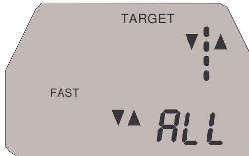
6. Momentarily press the AUD (audio) switch. The TARGET window will display “Aud” and a number from 0 to 5 indicating the audio level. With “Aud” displayed, press the RNG (range) switch until level 3 or 4 is displayed. Also, with “Aud” displayed, press the MODE switch, which will unscquelch the audio.
