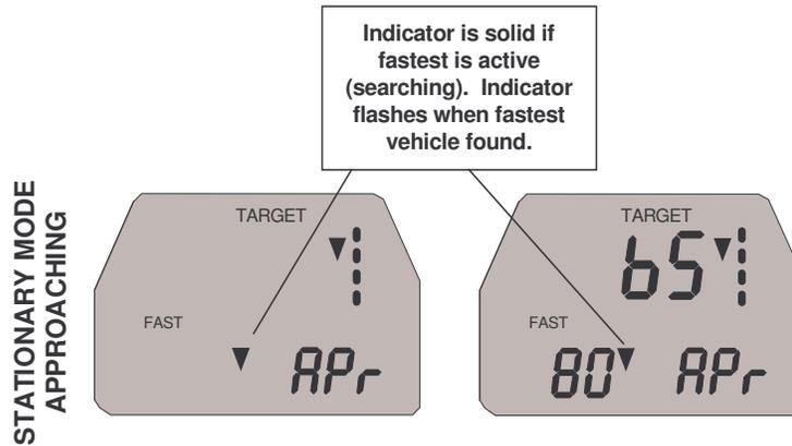
To activate the stationary, approaching targets only mode, repeatedly depress the MODE switch until “APr” appears in the PATROL window.
