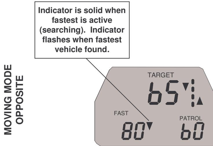
When operating the radar in Moving Opposite mode, the patrol vehicle and moving opposite road indicator will be on solid and the strongest vehicle speed will be displayed in the TARGET window.
