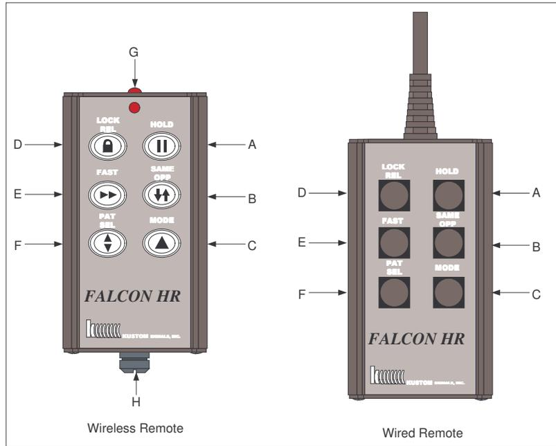
When the FalconHR has a handle attached and is placed in the mount, certain functions can be controlled with the Wireless/Infrared (IR) remote. If the unit is attached to the optional pod, a wired or IR remote can be used.
