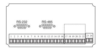
\* 8 VDC Power supplied on Pin 9 to power modem
