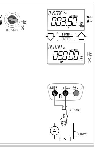
5.7.5 Alternating Current Measurement with Current Clamp Transformer, A AC and Hz  $\,$
