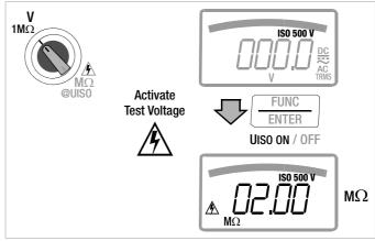
Auto-ranging is active during insulation resistance measurement.
