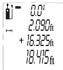
Fig. 7. A display showing the addition of a 16.325 ft. measurement to a measurement of 2.090 feet
