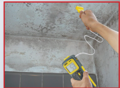
Pinned extension cable simplifies conventional measuring
