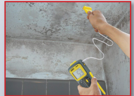
Pinned extension cable simplifies conventional measuring
