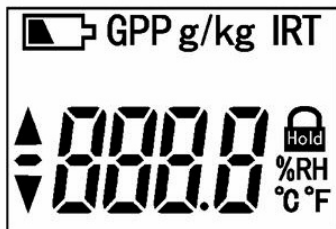
Fig. 1b. All possible display indications on the HT50
