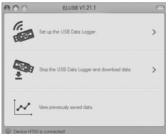
Fig. 2. The three options made available by plugging the HT50 into a USB port
