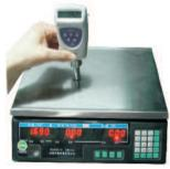
Apply a force N to the tip. When readings are almost unchanged, press the key 'MAX' to hold the reading P which should satisfy the equation below.
