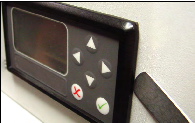
Figure 15: Checking the Gasket Compression
