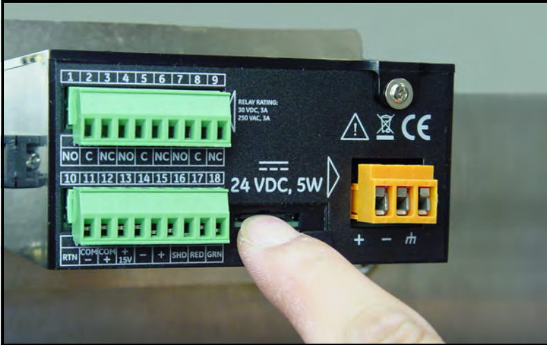
Figure 53: Pushing in on the MicroSD Card
