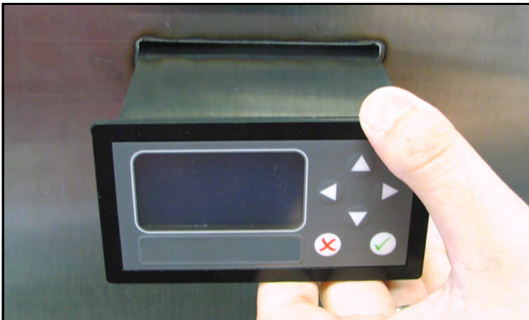
Figure 11: Sliding the Hygrometer into the Panel Cutout
