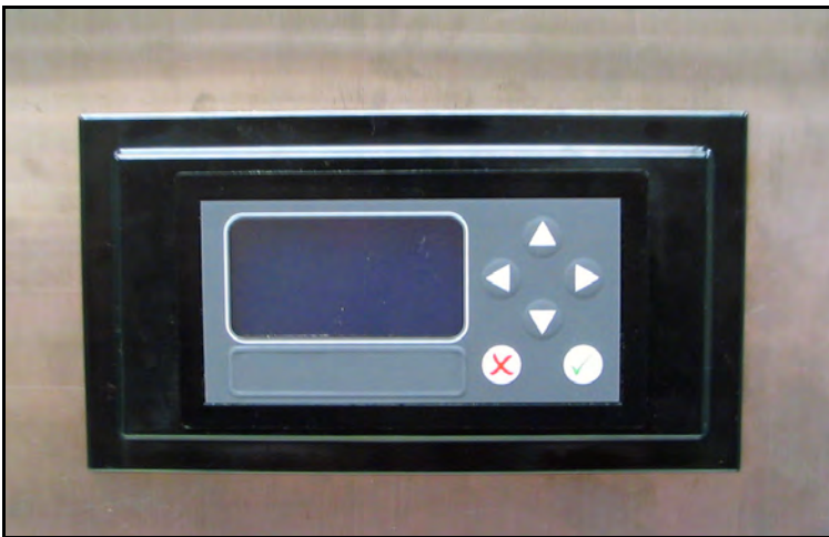
Figure 22: Hygrometer Installation with Adapter Plate - Front
