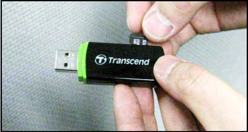
Figure 55: Plugging the Reader into a PC
