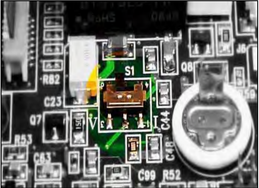
Figure 8: Switch S1 on the Main PC Board
