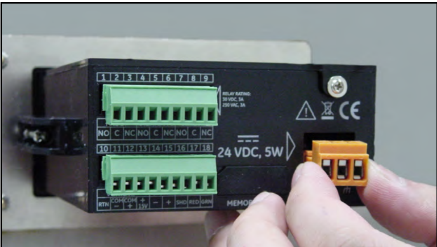
Figure 41: Removing the DC Connector
