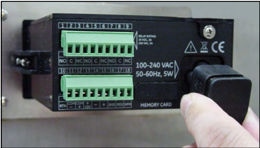
Figure 38: Inserting the AC Power Cable
