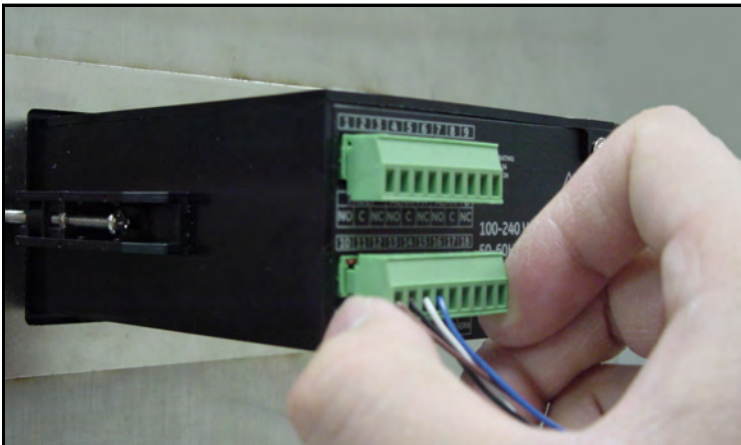
Figure 36: Reinserting the Connector into the Terminal Block
