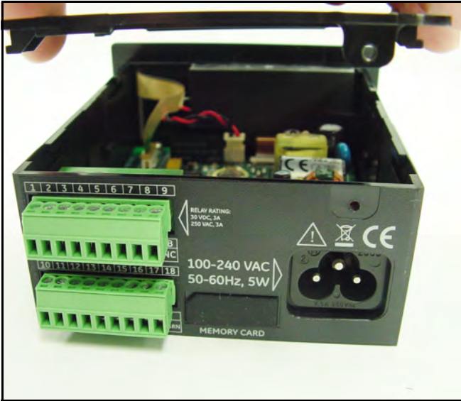
Figure 7: Lifting the Cover
