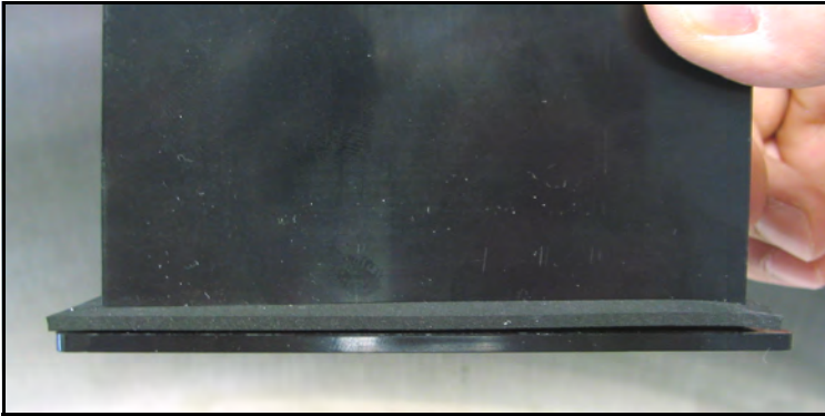
Figure 10: Installing the Gasket Behind the Display
