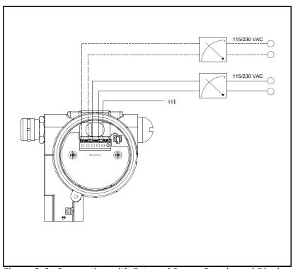
Figure 2-6: Connection with External Power Supply and Display
