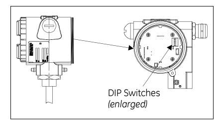
**4.** Use a pointed object (e.g. a screwdriver) and set switches 1-3 according to the desired output unit (see Table 2-1, below). Switch No. 4 has no effect.
