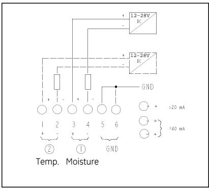
Figure 2-4: Connection with One or Two 24 VDC Power Supply
