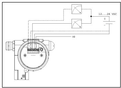
Figure 2-5: Connection with One 24 VDC Power Supply
