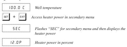
To exit out of the secondary menu press and hold the "EXIT" button. To continue on to the proportional band setting function press "SET".
