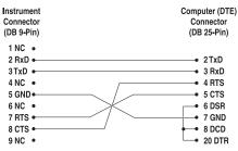
Figure 5 Serial Cable Wiring
