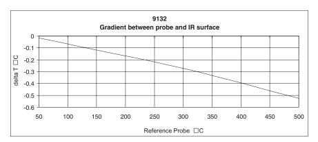
Figure 1 Temperature Gradient Between Probe and IR Target Surface
