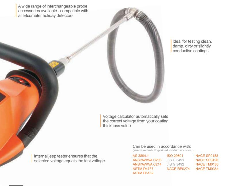
he Elcometer 280 uses the high voltage pulsed DC technique to detect holidays in coatings - even if the coating is damp, dirty or slightly conductive.
