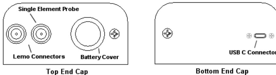
The top & bottom end panels are where all connections are made to the **ZX-6 DL**. The diagram above shows the layout and description of the connectors:
