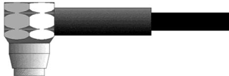
The Transducer is the “business end” of the **ZX-6 DL**. It transmits and receives ultrasonic sound waves that the **ZX-6 DL** uses to calculate the thickness of the material being measured. The transducer connects to the **ZX-6 DL** via the attached cable, and two coaxial connectors. When using transducers manufactured by Dakota Ultrasonics, the orientation of the dual coaxial connectors is not critical: either plug may be fitted to either socket in the **ZX-6 DL**.
