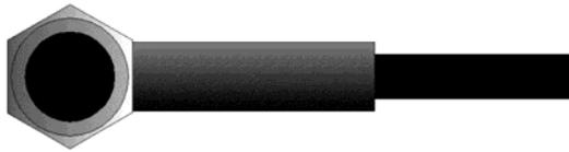
This is a top view of a typical transducer. Press against the top with the thumb or index finger to hold the transducer in place. Moderate pressure is sufficient, as it is only necessary to keep the transducer stationary, and the wear face seated flat against the surface of the material being measured.
