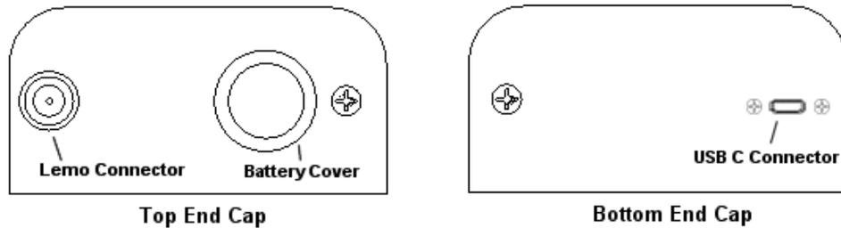
The top end cap is where all connections are made to the **PZX-7**. The diagram above shows the layout and description of the connectors:
