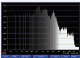
The FFT spectrum of the input signal is calculated at 1024 discrete frequencies.
