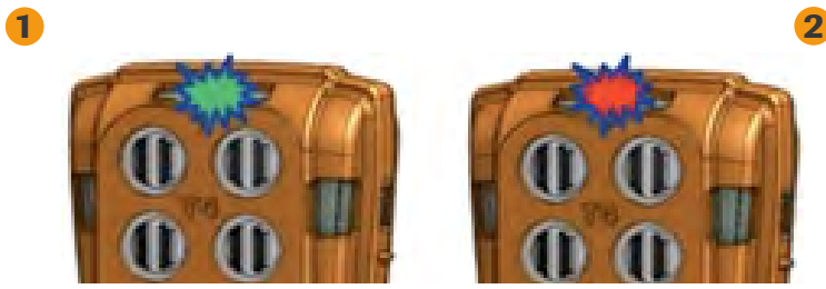
Figure 3: Battery Charge Status
