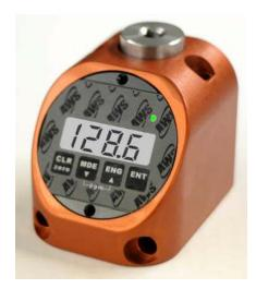
Press any Key to turn the unit on. Press CLR and ENT simultaneously to turn the unit off.
