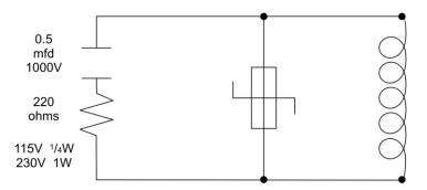
**Contacts:** - Arcing may occur across contacts when they open and close. This results in electrical noise as well as damage to the contacts. Connecting a properly sized RC network can eliminate this arc.
