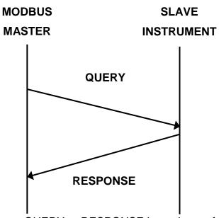
A message for either a QUERY or RESPONSE is made up of an inter-message gap followed by a sequence of data characters. The inter-message gap is at least 3.5 data character times - the transmitter must not start transmission until 3 character times have elapsed since reception of the last character in a message, and must release the transmission line within 3 character times of the last character in a message.
