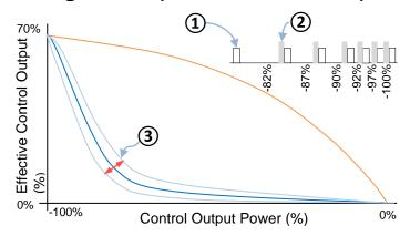
With non-linear cooling, e.g. when using water, the initial cooling effect can be stronger. For example, a change from 0% to -10% output power has more effect than say -70% to -80%. To compensate the cooling curve adjusts the output power so that the effective power over 0% to -70% is weaker.
