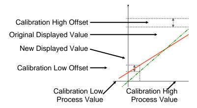
This example shows a positive Low Offset and a negative High Offset. For example:
