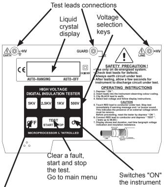
Reset ( if depressed for less than one second ) switches "OFF" the instrument when depressed for more than five seconds.
