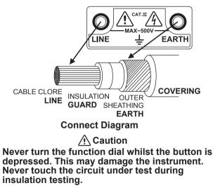
When testing is complete ensure that the TEST switch is released before the test leads are disconnected. This is because the system may be charged up and it must be allowed to discharge through the instrument's internal discharge resistor.
