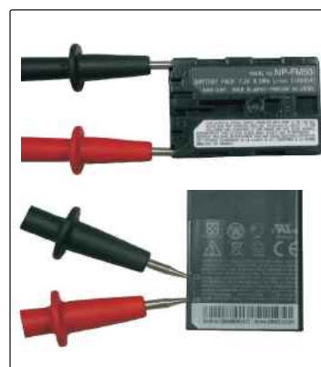
Li-ion Battery Measurement
