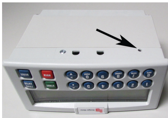
Figure 4: Grounding location, bottom view
