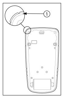
Figure 6. Front Shell Seal
