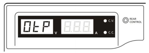
Figure 9 - Overtemperature Protection
