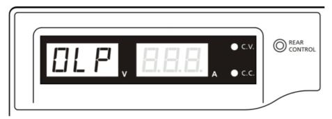
Figure 10 - Overload Protection
