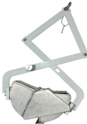
Easily sample most types of bottom surfaces. The top of the sampling chamber is screened to allow water flow during deployment and reduce the frontal shock wave that may displace sediment as the dredge contacts the sample surface.
