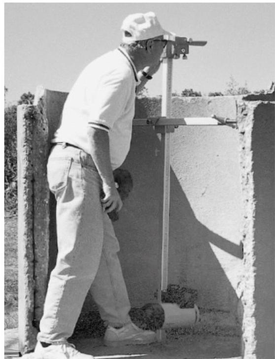
3. Align Transit to Laser – Tilt the transit down and sight on the line pivot LED. On the transit, use the laser centerline knob to adjust the vertical crosshair until it is exactly aligned with the line pivot LED on the laser. Repeat steps 2 and 3 until the crosshair is on the forward manhole marker and the line pivot LED.
