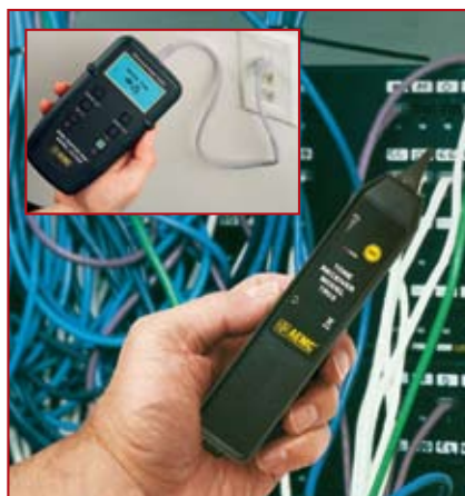
Model TR03 used to find cables in a panel.
